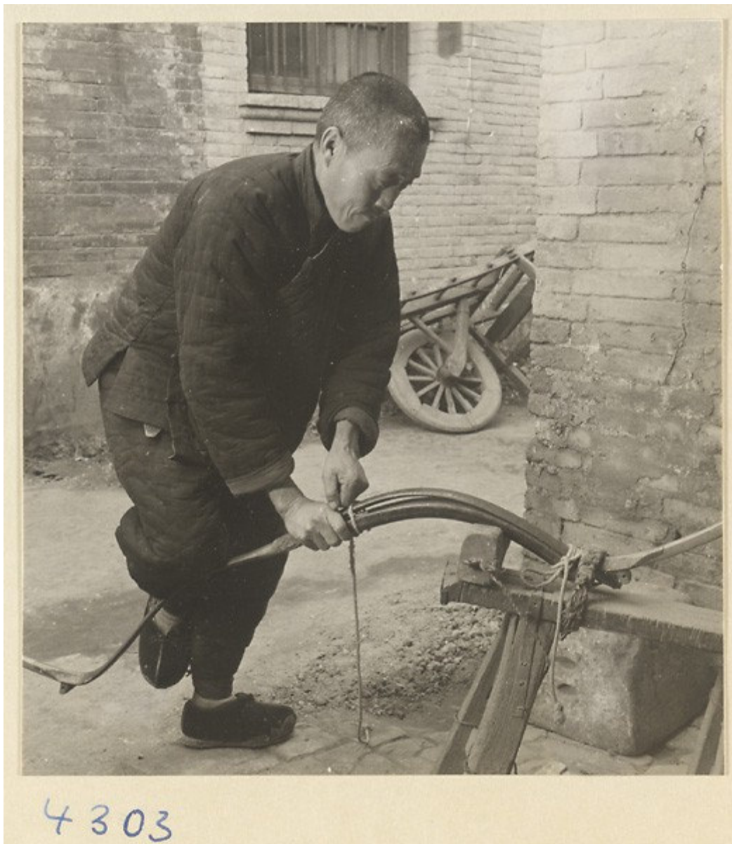
Bending one bow limb over a bending block, or gong nazi . Heavy Manchu bows are really hard to string and using this method you pre-bend the limbs so that the stringing process is made easier for the handler and less risky for the bow.
