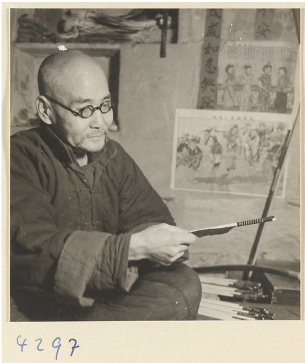
Putting the feather on the shaft. Timing is very important here, letting the hot glue not cool down too much before letting the surfaces touch.
