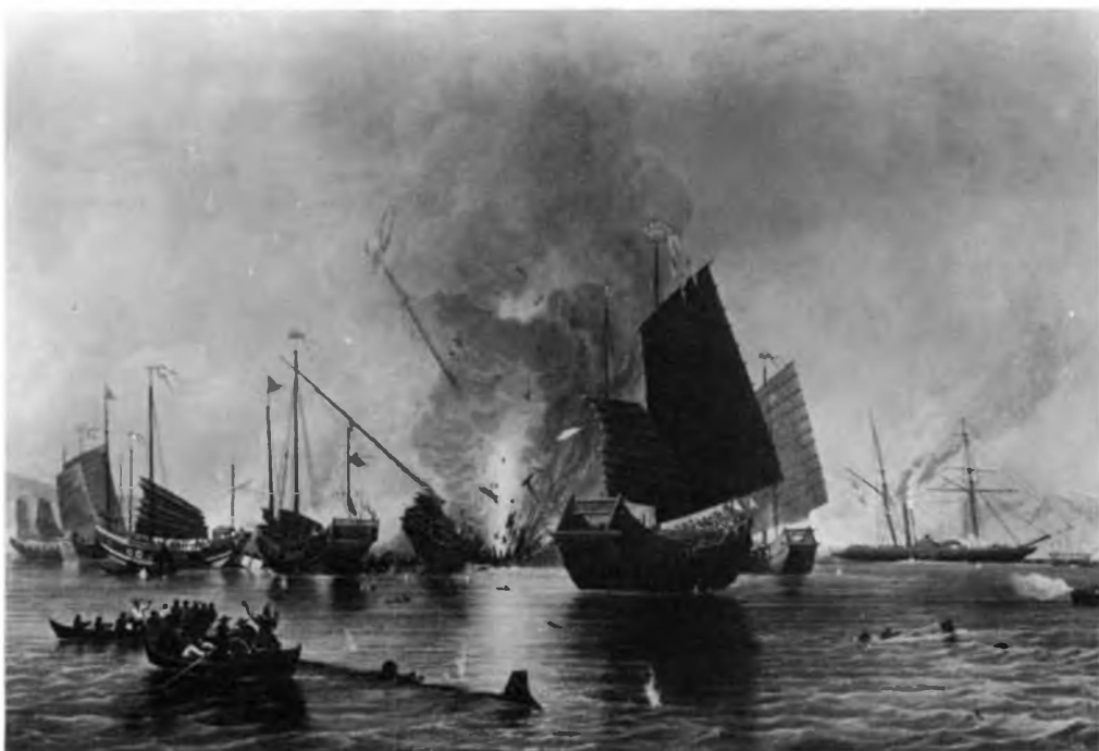
The "Nemesis" (right) During the Opium War the Nemesis , an uncoppered paddle-wheel iron ship that operated by sail or steam, proved effective for the British in the campaigns off Canton and Shanghai.
