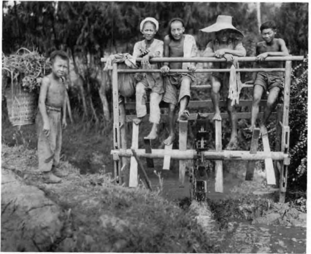
Pumping water, An Chu Chang, 1917 (photograph by Sidney D. Gamble) The irrigation of fields with water wheels such as this was a centuries-old practice in China.
